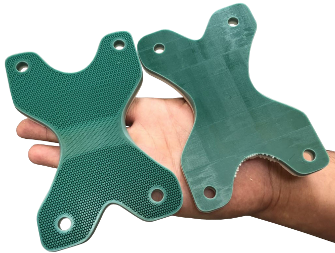
Figure 6: Example Cross Section of Sparse Infill Mode on ProJet 2500 IC
