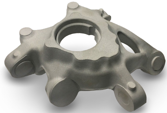
Figure 11: Final Cast Part
